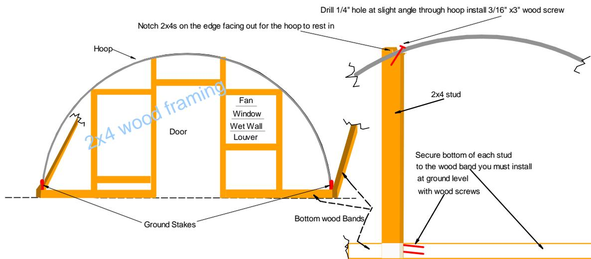
Typical wood stud end wall framing, Number of studs required are variable subject to house size and uses.
