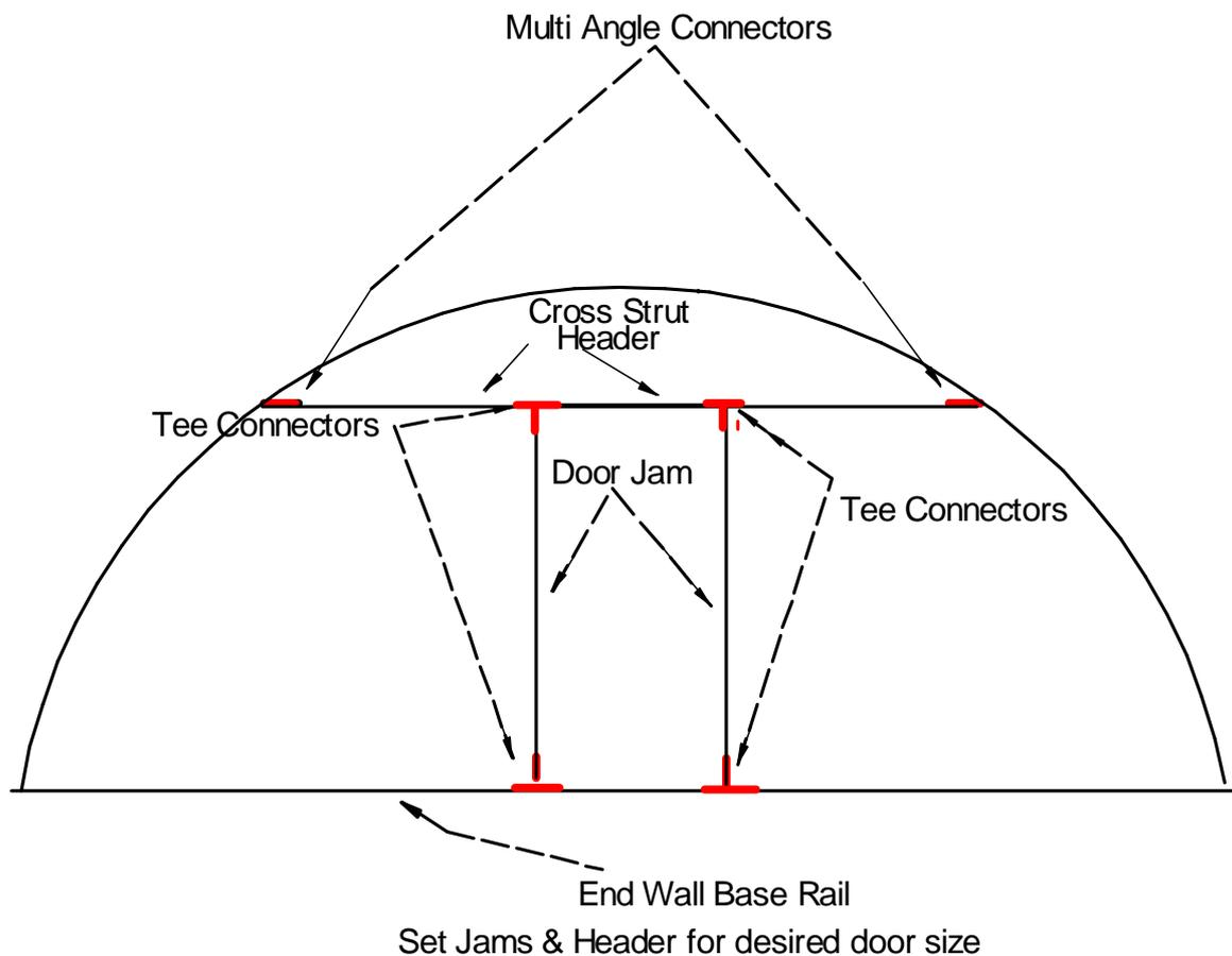
This can also be used for lighter weight 1" emt hoop movable & anchored hoop houses , just purchase same welded connectors for the 1" emt size instead of 1 3/8". Please NOTE that split tees are not available for 1" emt, only the welded connectors are available for 1" movable or anchored.
