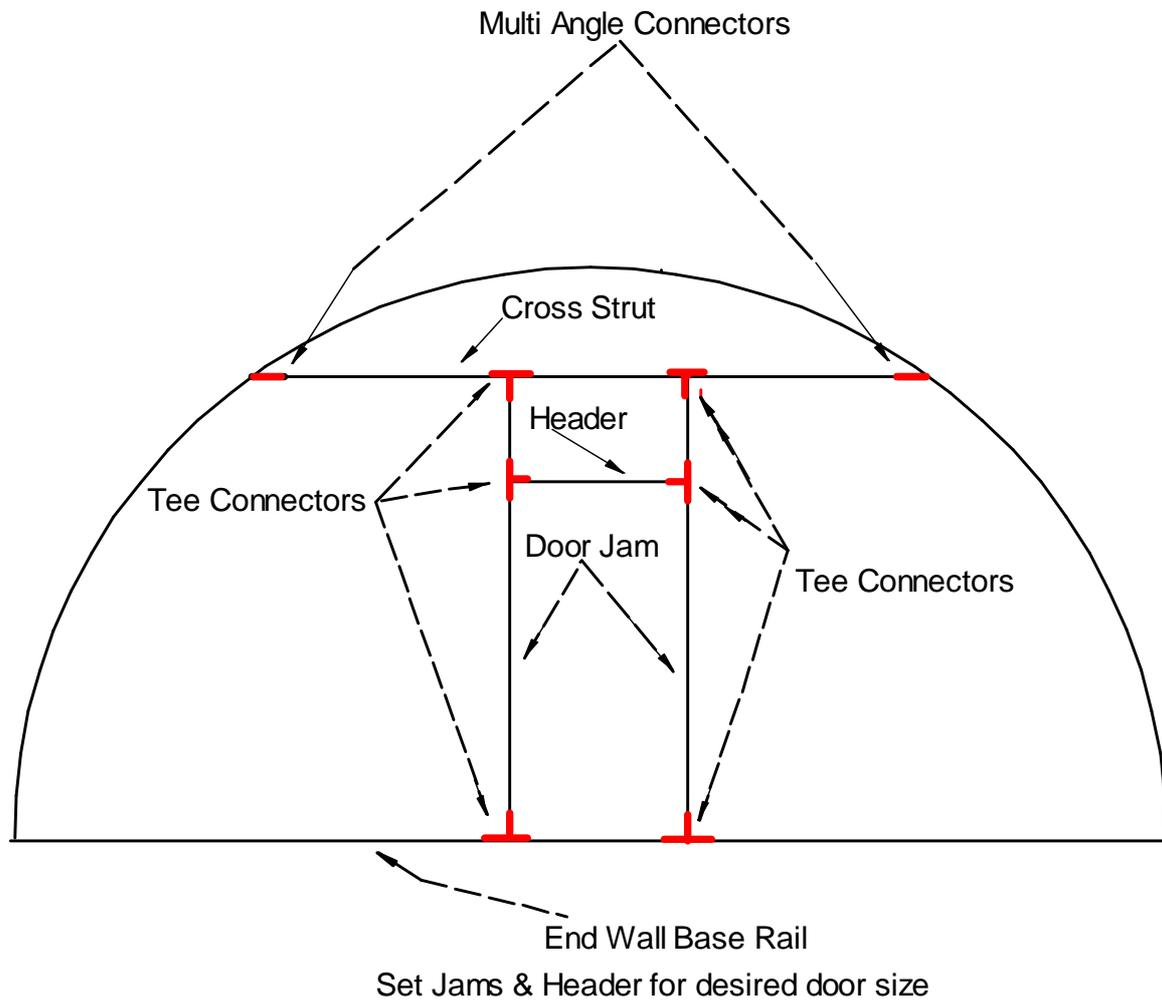
This can also be used for lighter weight 1" emt hoop movable & anchored hoop houses , just purchase same welded connectors for the 1" emt size instead of 1 3/8". Please NOTE that split tees are not available for 1" emt, only the welded connectors are available for 1" movable or anchored.
