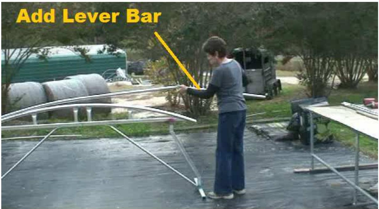
**Pull down until the junction of lever bar & tube touch bender**
